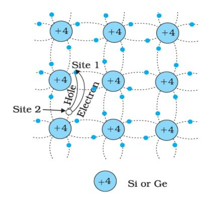
Simplified representation of possible thermal motion of a hole
