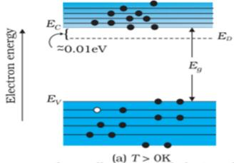
one thermally generated electron-hole pair + 9 electrons from donor atoms
