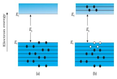
Fig (a) shows an intrinsic semiconductor at 0K and since there are no electrons in the conduction band it behaves like an insulator
