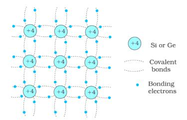
Schematic two-dimensional representation of Si or Ge structure showing covalent bonds at low temperature (all bonds intact) +4 indicates inner cores of Si or Ge.Figure schematically shows the 2-dimensional representation of Si or Ge structure. This is the figure you usually draw in your notebooks to show covalent bonds.
