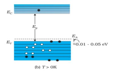
• The acceptor energy level E<sub>A</sub> is slightly above the top E<sub>v</sub> of the valence band as shown in figure.
