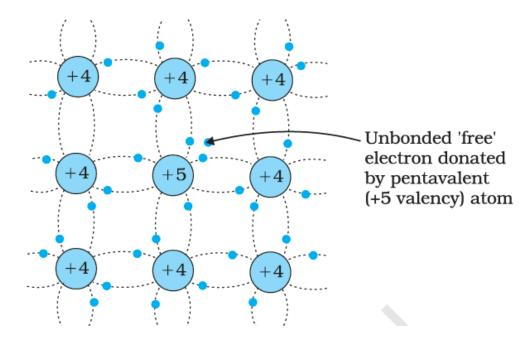
When an atom of + 5 valency element occupies the position of an atom in the crystal lattice of Si, four of its electrons bond with the four silicon neighbours while the fifth remains very weakly bound to its parent atom. This is because the four electrons participating in bonding are seen as part of the effective core of the atom by the fifth electron.
